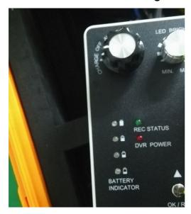
3. The battery is been charged. You can see the charge adaptor light is "Red" color. When the battery is charged "full", the LED light will be "Green" color.
