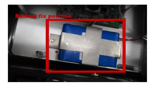
Fourth: Connect battery cable with mainboard port, as below picture
