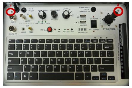
**Second:** Remove the control box keyboard, then you can see these screws,(as below picture), remove these screws.
